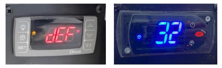
If you notice that your case is running warm but not in defrost, check the filter for any build-up as well as the case vents for blockage or debris.
