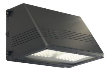
**CONSTRUCTION:** Precision die-cast aluminum housing with stainless steel hardware, tempered borosilicate glass refractor and ingress resistant gasket. Knock-out on housing for available button photocell accessory
