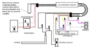
2. Wiring If Power Of Luminaire ≤power Of Led Emergency Driver.
