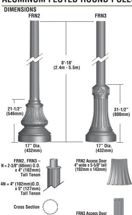
**POLE SHAFT** - The pole shaft is either spun or extruded from 6000 series alloy aluminum. Tenon N option is 2-3/8" O.D. x 4" tall. Tenon 4N option is 4" O.D. x 5" tall. Aluminum 16 flat fluted round pole shafts with decorative base are 4", 5" and 6" in diameter. Poles have a cast ring between shaft and tenon.
