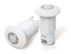
The AirLink Blue ceiling motion and daylight harvesting sensor provides wireless lighting control based on motion and available ambient daylight. Multiple fixtures can be grouped to be controlled by a single ceiling motion and daylight harvesting sensor. Controls 0-10 VDC LED drivers and is rated for indoor installations. Ceiling motion and daylight harvesting sensor utilizes a Bluetooth Low Energy (BLE) mesh network. Dim levels and schedules can be set through LSI AirLink Blue iOS app.
