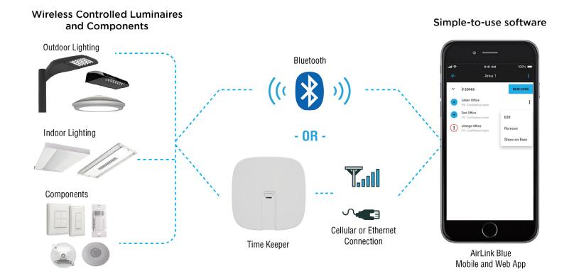
AirLink Blue ships can be configured to the owner's requirements via a web and mobile app. Changes or updates to the control system can be accomplished on site via iOS smart phone app.
