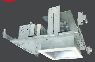
4 inch LED new construction downlight delivers superior performance and energy efficiency. Designed to use anodized aluminum reflectors delivering even illumination and low glare. The high performance luminaire offers a 2000 lumen package with color temperatures of 3000K, 3500K, 4000K at 80 CRI. Standard driver offers universal (120-277V) and 0 -10V dimming down to 1%. The LAD series is ideal for low to medium ceiling heights for retail, hospitality and commercial applications.
