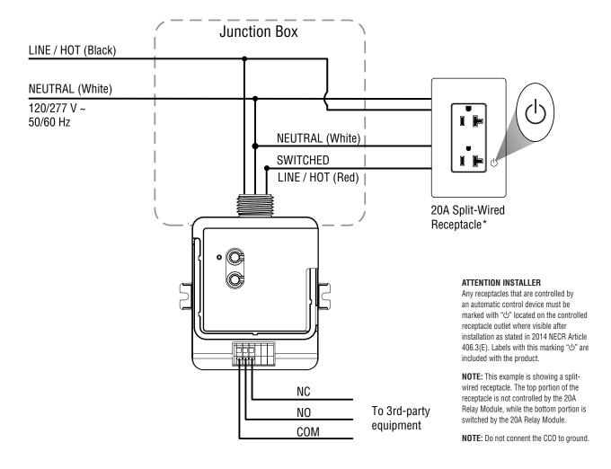
NOTE: Some applications (in USA) require the module to be installed inside an additional junction box.
