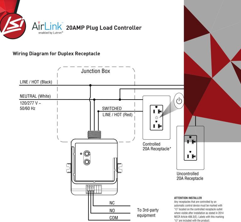
**NOTE:** Some applications (in USA) require the module to be installed inside an additional junction box.
