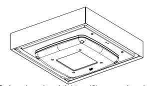
Swing closed and tighten (2) screws/toggles Make sure screw toggles are fully engaged on inside of rim!
