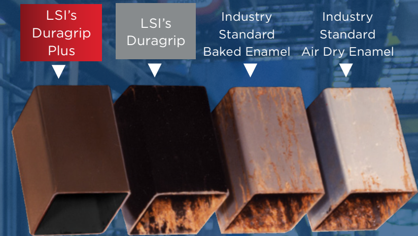
Poles After 1000hrs of Salt Spray Test
