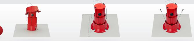
Slide the locking collar over the capsule. Align the REDiMount to a rib on the canopy using a square. Secure the four screws into the capsule making sure to use between 25-35 inch-pounds of torque. Repeat this process on top of the canopy with every fixture.
