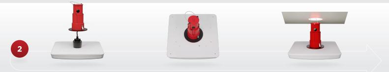
Plug in quick connect, push down and lock on capsule to the luminaire. Drill a 4" hole into the mounting location of the canopy; Lift or hoist the luminaire with connected REDiMount using the affixed hoist strap up to the canopy.
