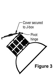
1. Remove Luminaire wiring box cover by removing the cover end screw. Swing the cover up and off the pivot hinge.
