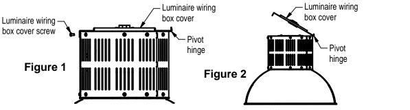
Secure cover to J-box (not suplied) with suitable screws (not supplied). Note orientation and position, so that it will re-connect to Luminaire. Use all (4) slots in cover to attach J-box. Hang Luminaire onto Cover, so that it suspends from the pivot hinge. See Figure 3.
