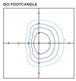
15' Mounting Height/15' Grid Spacing 5 FC 2 FC 1 FC 5 FC POLAR CURVE
