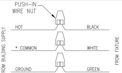
\* FOR 220/240/480V THE COMMON WIRE IS REPLACED WITH HOT.
