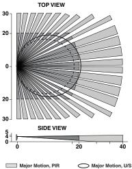
Provides a 180° field-of-view with a maximum coverage area of approximately 2400 square feet. The maximum major motion sensing distance in front of the sensor is 40 feet, and side to side is 30 feet. The "minor-motion" zone detects relatively small body movements and allows the lights to stay ON even though a person may not be moving or walking around the room. This zone is approximately 40 feet by 20 feet.
