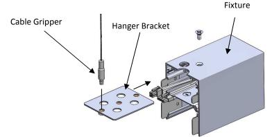
Use provided flathead screws to secure hanger bracket to fixture.
