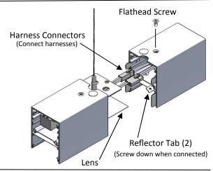
Tuck in harness at the end of rows and attach endcaps using supplied screws.
