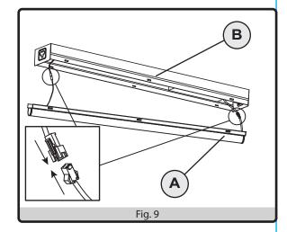
10. Snap the LED cover assembly (A) back onto the housing base (B) to complete the installation.
