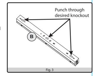
4. Align knockout hole with the supply wire location on the mounting surface and hold the housing base (B) up in its intended location with one hand while marking the location of the two keyhole slots at each end of the fixture plate.
