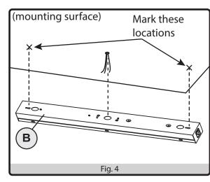
DRYWALL MOUNTING: If the mounting holes go through drywall without a stud, drill four small pilot holes using a 1/8-in. drill bit (not included), and install drywall anchors (BB) into the holes with a hammer (not included).
