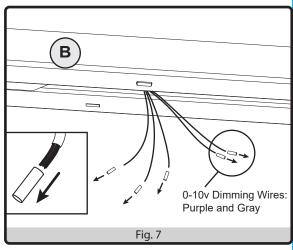
8. Connect the fixture wires to the supply wires -black to black, white to white, and green to
