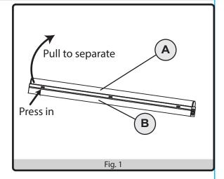
2. Locate the wiring quick disconnect connectors between the two halves and release the connectors to separate the wires between the two halves. Set aside the LED cover assembly (A).
