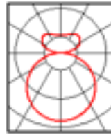
30/70 - Option 3415 lumens 33% up - 67% down 80 lm/W
