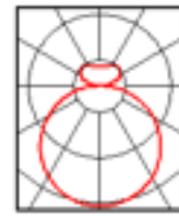
20/80 - Option 3285 lumens 22% up - 78% down 75 lm/W
