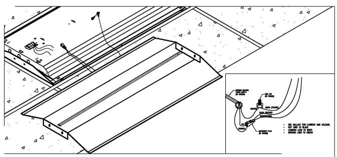
5.) attach ground wire to existing housing using tek screw. This will provide ground continuity as well as a tether to assist in installation.
