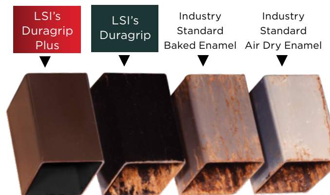
Poles After 1,000 hours of Salt Spray Test
