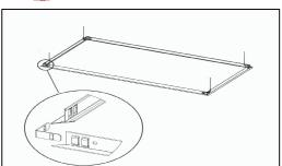
FK: Designed to be used with any grid type recessed luminaire in ceiling requiring flanges. May be nailed to framing for purpose of trimming out the ceiling opening not to be used for support of lumimaire. If this method of installing FK is used luminaire must be supported by #12 ga. mild steel wire by others.
