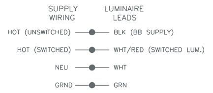
19. Luminaire is supplied with a fuse attached to outside of housing. Install fuse in fuse holder AFTER luminaire is mounted and supply connections are made. Fuse is required for proper emergency operation. See separate installation instructions supplied for Battery backup unit.
