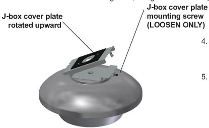
4. Loosen J-box cover mounting screw (do not remove). Slide and rotate J-box cover plate
