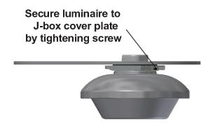
10. Making sure no wires are in the way or pinched, swing luminaire up evenly with J-box cover plate. Secure luminaire to plate by tightening screw on luminaire. This completes installation of XNPG D.
