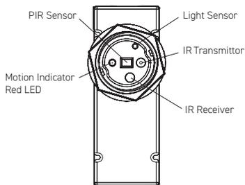
The IMS is a motion sensor that dims lighting from high to low based on movement. This slim, low-profile sensor is designed for installation inside the bottom of a light fixture body. The PIR lens module connects to the IMS through a 1.30" diameter hole in the bottom of the fixture.
