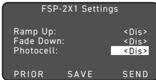
When the light level exceeds this setting, the lights will turn off even when the space is occupied. Once the light level exceeds this setting, the sensor will
