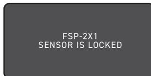
This screen will appear if the sensor is locked. If it is locked, cycle the power.
