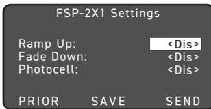
Time period for light level to increase from LOW to HIGH (default is Disable; light/load switches instantly).
