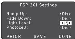
Displays the light level at the sensor. The light level reading can be used as a reference for setpoint adjustments.
