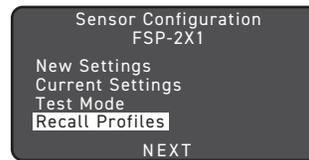
Recall Profiles allow the user to select the saved parameter profiles. This feature is used when programming multiple Sensors with the same parameters.
