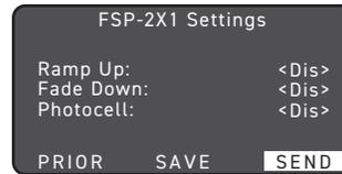
To program the sensor with the selected parameters go to SEND and press the Select button. The controlled load should cycle once the sensor is updated.
