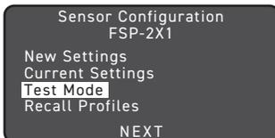
Test Mode shortens timeouts for High/Low and Cut Off, to allow quick verification of settings. Test Mode disables automatically after 5 minutes.
